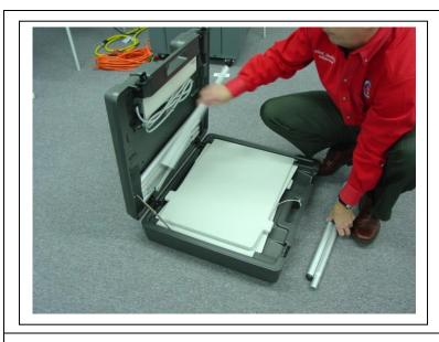
5. Open lid and remove four individual legs and one four-leg assembly.
